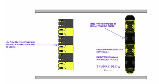
TRAFFIC FLOW CONTROL PLATES ARE DESIGNED TO ENCOURAGE ONE WAY TRAFFIC FLOW AND PREVENT UNAUTHORISED ENTRY/EXIT WITHIN ANY LOCATION.
